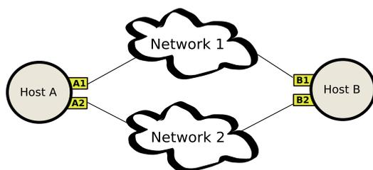
Fig. 1. Example of multihoming (with disjoint paths).
