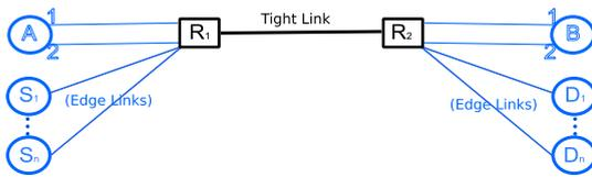
Fig. 9. Simulation topology for the TCP-friendliness of CMT.
