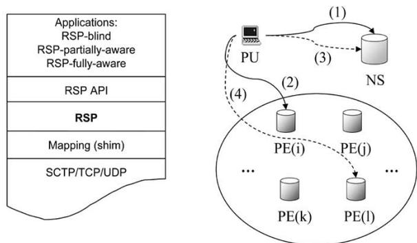
Fig. 1. Reliable server pooling: protocol stack and basic operations.
